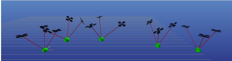
Figure 9: Collection of 5 snapshots along 3 Quadrotor 1 Mass system trajectory.
