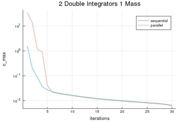
Figure 3: Maximum constraint violation during solve for 2 Double Integrators and 1 Mass system.
