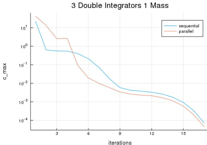
Figure 5: Maximum constraint violation during solve for 3 Double Integrators and 1 Mass system.
